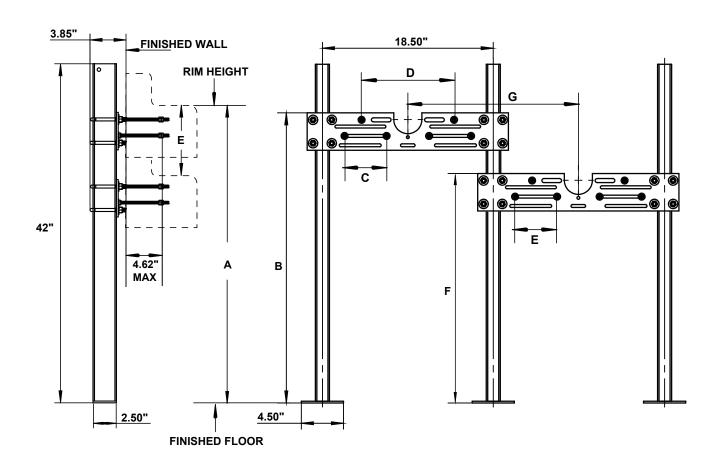
Recommend all feet to be secured to floor with 1/2" bolt and anchors
