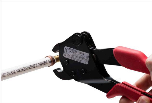
3. Position ring over sealing barbs of the fitting. The ring should be positioned approximately 1/8" to 1/4" from the end of the tube.
