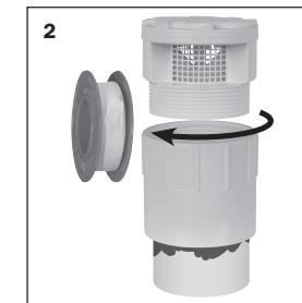
Apply PTFE tape to threads on TurboVent. Screw into adapter. Do not use tools or pipe dope.
