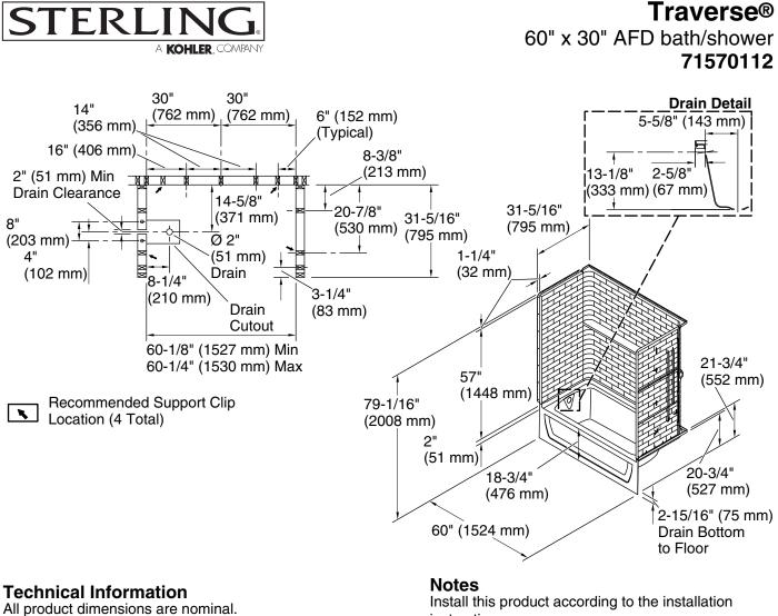
Installation: Three-wall alcove Maximum door 58-3/4" (1492 mm) height: Maximum door 57-5/8" (1464 mm) width:
