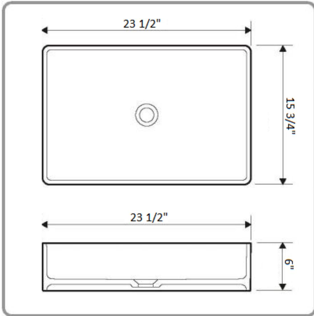
**This sink does not have an overflow. Use with our P0661 lav sink drain.**
