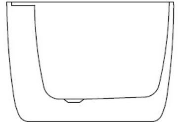
**The Overflow channel is molded into the interior tub wall. Drain is included.**
