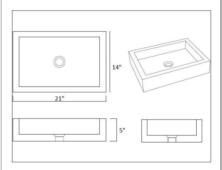
This sink does not have an overflow. Use with our P0661 lav sink drain.
