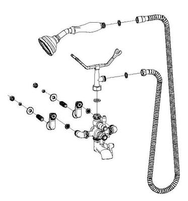
This faucet is tested to remain within 1 degree Fahrenheit of your desired setting throughout its operation, with an automatic temperature stop at 104 degrees Fahrenheit. The unit also has a built-in anti-syphon.
