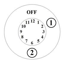
"1" opens LEFT outlet Shared Function between outlet "1" and "2" "2" opens RIGHT outlet
