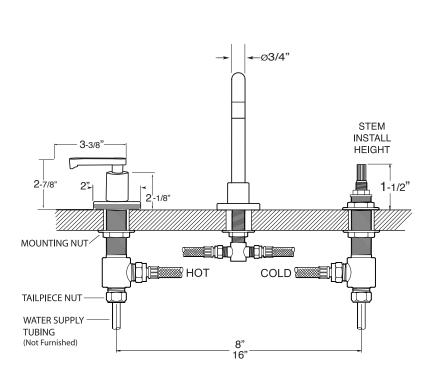
NOTE: Spout and valves install through 1-1/4" diameter holes
