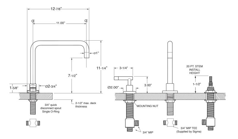
NOTE: Spout and valves install through 1-1/4" diameter holes. Plumber to provide 3/4" supply lines to valves
