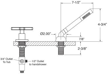
Spout and valves install through 1-1/4" diameter holes.
