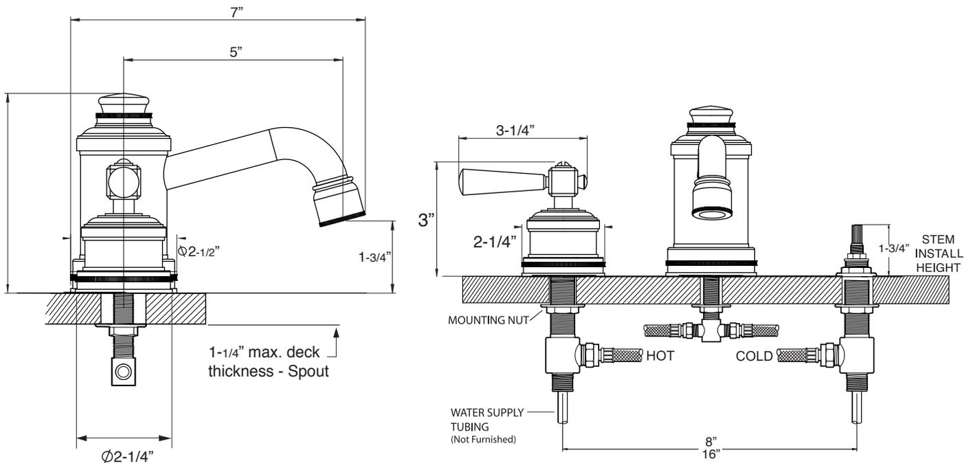
NOTE: Spout and valves install through 1-1/4" diameter holes
