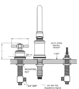
NOTE: Spout and valves install through Ø1-1/4" diameter holes.
