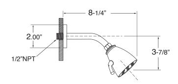
Note: See installation Instructions for length of stem required from finished wall.
