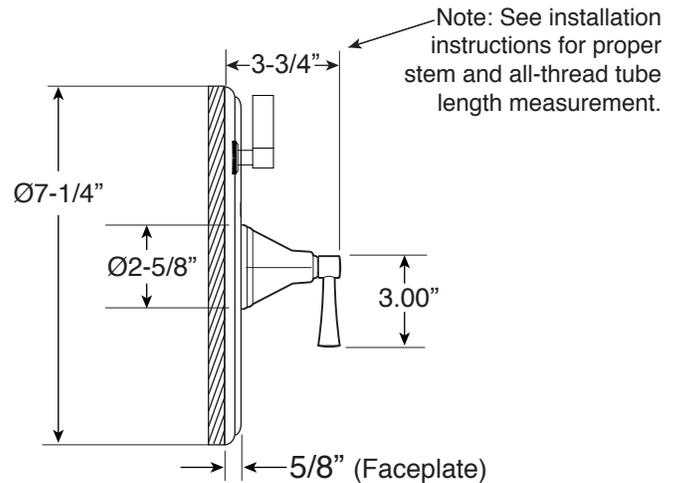
Note: See installation instructions for proper stem and all-thread tube length measurement.
