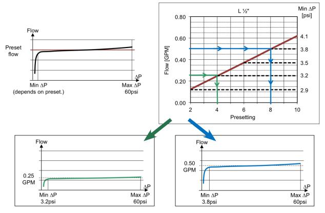
The flow regulating assembly determines the stroke length. When coupled with a modulating actuator, the control signal and the actual output flow is proportional (example for a RWV actuator with control signal 0-10V). In the above example, at 0.5 GPM a presetting of 8 is determined on a L  $\frac{1}{2}$ " valve. The valve will start to operate at a  $\Delta P$  of 3.8 psi.
