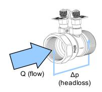
Formula linking flow Q (in GPM) and theoretical valve headloss  $\Delta p$  (in psi).
