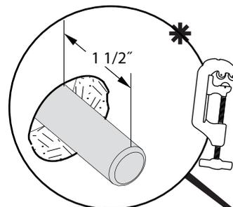
\* Cut the Slip-Fit Shank 1 1/2" long from the finished wall and remove any burr's before installing the Wall Spout.
