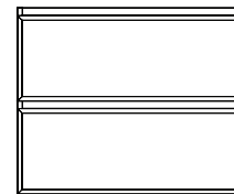
Two H2 - 15" (381 mm) Profiles vanities stacked Total height 30" (762 mm)
