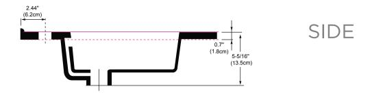
By IAPMO, ceramic lavatory warpage is defective only if warpage of flat slab out of horizontal plane exceeds 6.3 mm/m (0.25 in/ft) on all sizes OR warpage on back of lavatories that are attached to the wall exceeds 3 mm (0.13 in).
