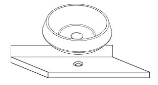
**Step 2:** Place a generous portion of plumbers' putty under drain cap and insert whole drain body inside the bowl and through the countertop.
