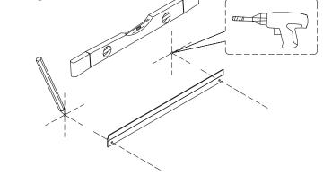
**Step 3:** Secure the wall cleat to with the long screws provided.
