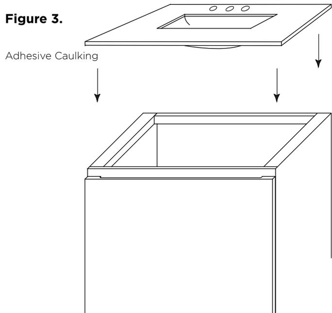
**STEP 3:** Secure top & back splash to cabinet by using adhesive caulk
