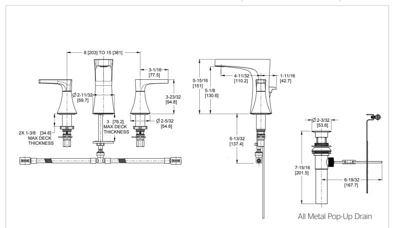
Ø1-1/4 Min to Ø1-1/2 Max. Deck Hole Openings
