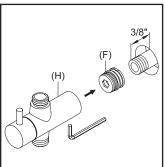
(1) Make sure the inlet is 1/2" pipe nipple and must protrude 3/8" from the finished wall.
