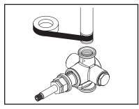
(1) Please refer the drawing in the bottom right to determine the distance to install valve to the recommended depth based on different finished walls. Improper installation may result in performance and aesthetic issue with the product. For IPS connection:-Apply Teflon tape on valve's inlet and outlet ports, make sure to identify which one is the inlet port of the valve, connect water pipes to inlet and outlet ports, cap the unused outlet port if there is any.
