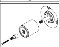
(2) Thread the sleeve on the valve. Install the handle adapter on the stem and secure the handle adapter with the screw.
