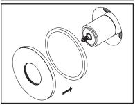
(3) Slide the face plate on the sleeve. Ensure the rubber gasket is behind the face plate. Apply silicone to caulk around the flange to form water tight seal.
