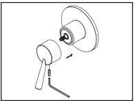
(4) Attach the handle to the handle adapter. Tighten the Allen screw to secure the handle by using 3/32" Allen wrench. Check if the water diverts to desired outlet properly.
