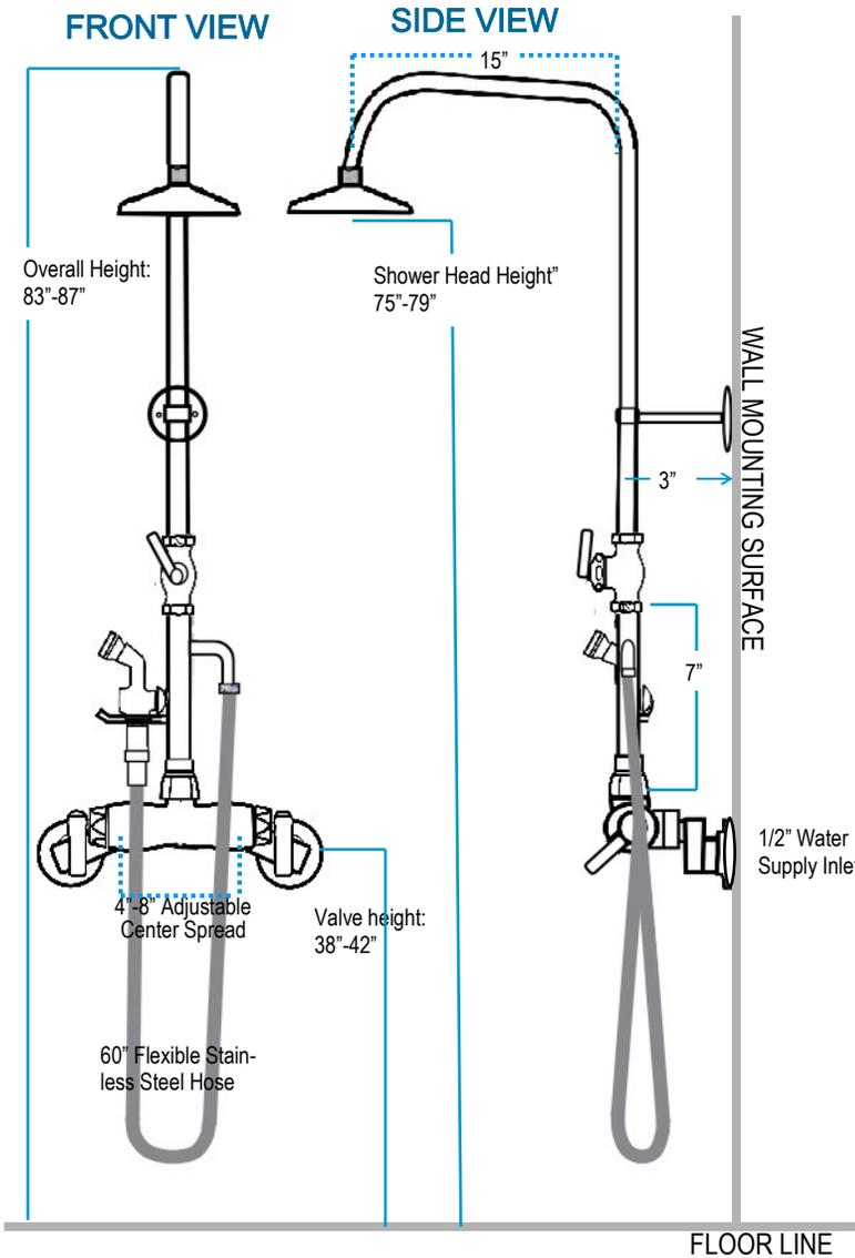
**NOTE:** Flush supply lines before installing valve to remove chips and dirt which can become lodged in the seat washer and cause the faucet to malfunction.
