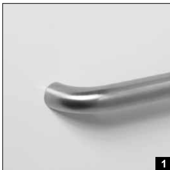
Photo 1: Grab Bars: Factory-installed 1.50-inch diameter, concealed attachment, 18 gauge, #304 brushed stainless steel grab bars. Concealed attachment design provides tamper-resistance and minimizes debris collection areas at contact points, compared to common exposed flange bar designs, without compromising bar attachment integrity. (Reinforced areas include a structural core material encapsulated in FRP composite.)
