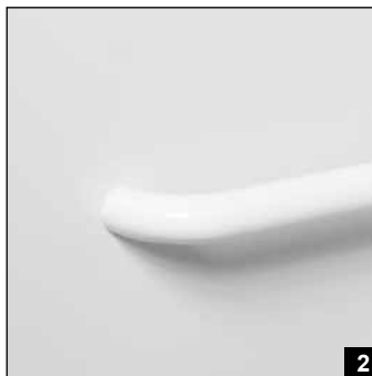
Photo 1: Grab Bars: Factory-installed 1.50-inch diameter, concealed attachment, 18 gauge, #304 brushed stainless steel grab bars. Concealed attachment design provides tamper-resistance and minimizes debris collection areas at contact points, compared to common exposed flange bar designs, without compromising bar attachment integrity. (Reinforced areas include a structural core material encapsulated in FRP composite.)
