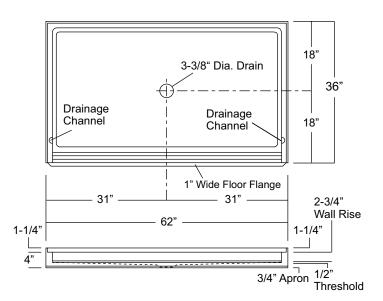
NOTE: Critical enclosure dimensions should be taken directly from the installed shower base with finished wall surround.
