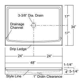
NOTE: Critical enclosure dimensions should be taken directly from the installed shower base with finished wall surround.
