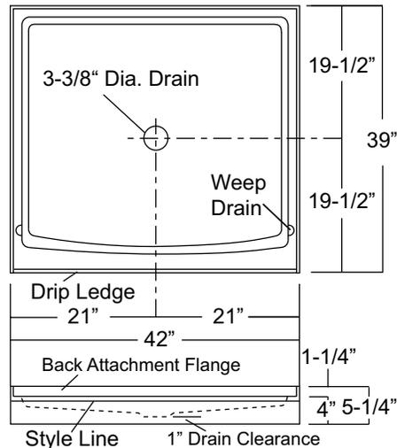
**NOTE:** Critical enclosure dimensions should be taken directly from the installed shower base with finished wall surround.
