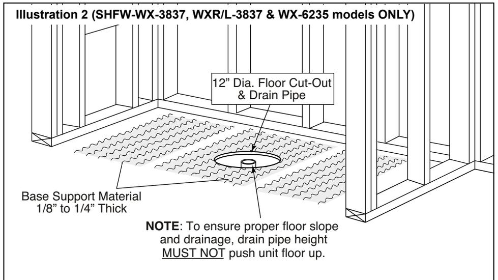
**NOTE:** To ensure proper floor slope and drainage, drain pipe height **MUST NOT** push unit floor up.
