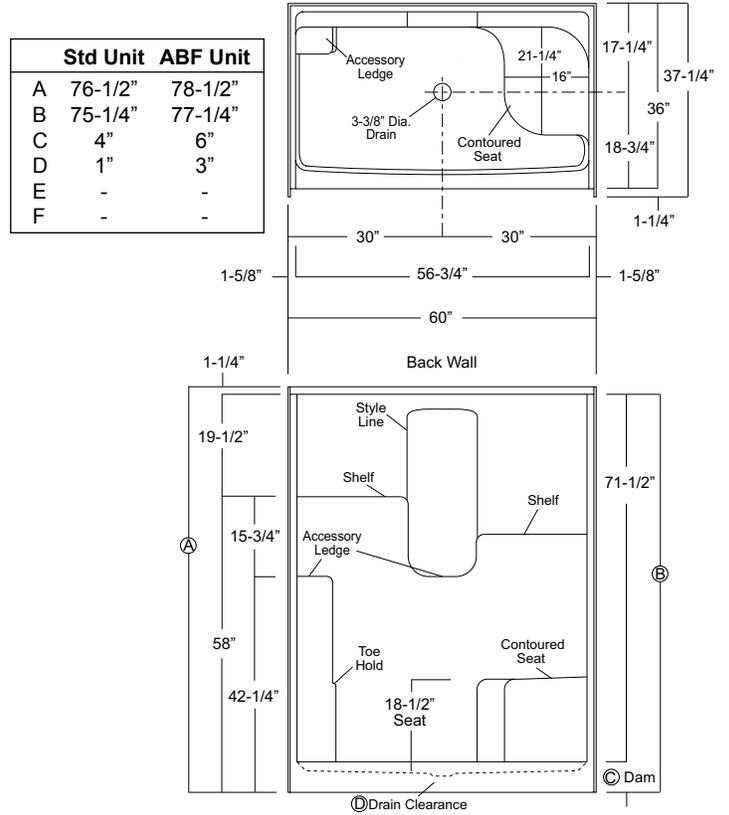
**Illustration 1c - Center Drain, Unit Dimension & Alcove Framing Guidelines (dimensional tolerance +0 / -3/8")**
