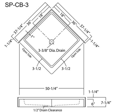
**Illustration 1b - Unit Dimension & Alcove Framing Guidelines (dimensional tolerance +0 / -1/8")**
