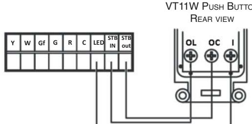
9. Plug the ventilation unit and test the wall control (A). The LED indicator will turn on to indicate that the unit is working. Push the button again to turn the unit OFF. **UNIT WILL REMAIN POWERED**, but will not work.
