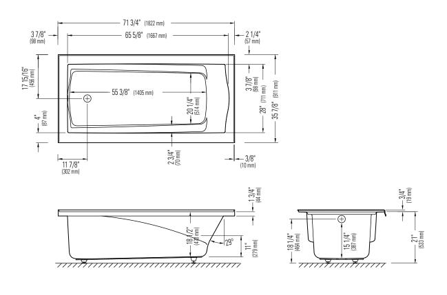
\*A bathtub fitted with back jets can cause the pump to protrude by approximately 3" from the overall dimension.
