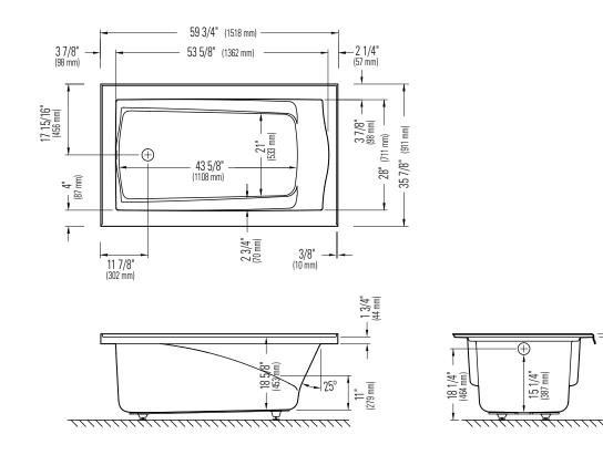
\*A bathtub fitted with back jets can cause the pump to protrude by approximately  $3^{\prime\prime}$  from the overall dimension.
