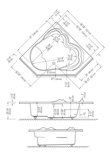
$<sup>^*\</sup>mbox{A}$  bathtub fitted with back jets can cause the pump to protrude by approximately 3" from the overall dimension.
