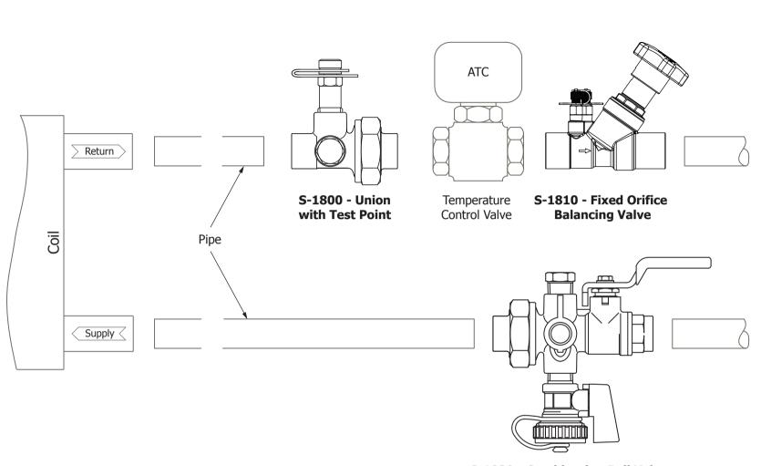
S-1830 - Combination Ball Valve with Drain and Test Point
