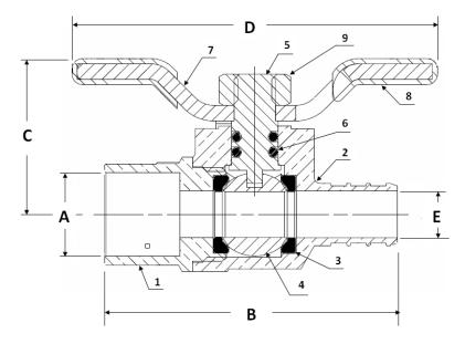
**Specifications:** Designed for residential, commercial or industrial use with water, oil or gas. This approved Webstone valve is actuated by a blowout proof stem. Solder joint temperature ratings are per ASME B16.18 Annex A for 95-5 solder. Other solder materials have lower pressure/temperature limits. Do not silver braze or overheat valves when soldering.
