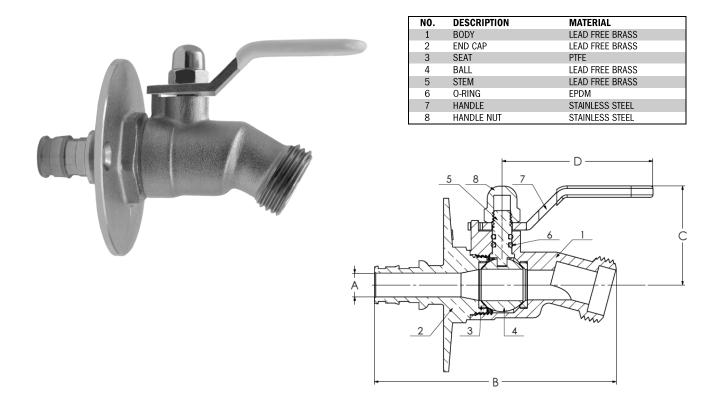
**Specifications:** 3320W Series Designed for residential, commercial or industrial use with water. Pex end dimensions are in accordance with ASTM F1960. This approved Webstone valve is actuated by a blowout proof stem. Threaded ends comply with ANSI B1.20.7
