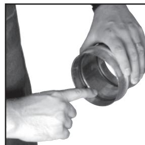
4. Check the fitting to make sure that the seal is in place and is free of oil or grease. Only original NIBCO EPDM seals are to be used when making a press connection with NIBCO Press System fittings and valves. If it is necessary to lubricate the seals, use water only. **DO NOT** use any petroleum-based lubricants.
