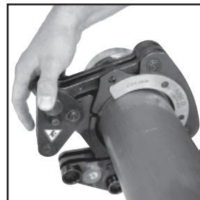
6. Select the correct size pressing chain. Pull the pin on the chain which allows the segments to open. Position the chain on the raised bead and wrap the chain around the fitting with the "pipe side" designation facing the tube. When the chain is fully wrapped around the fitting, reinsert the pin to secure the chain on the assembled joint. Visually inspect the mark made in Step 5 to ensure the tube remained in position.
