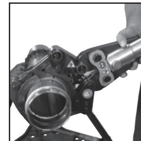
8. Squeeze adapter jaw arms to open the jaw. Rollers must be fully retracted to open the adapter jaw. Place the open adapter jaw into grooves in the pressing chain and let go of the jaw arms. Make sure the tube is inserted to the proper depth in the fitting (reference mark from #5). With the pressing tool perpendicular to the tube, begin the pressing cycle by pulling the trigger of the tool.
