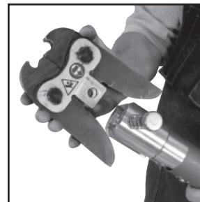
7. Release the pin (push and twist) on the jaw holder of the pressing tool, and install the adapter jaw on the tool. Return the pin to its original position, securing the jaw. The red sleeve on the tool must be in the back position to allow for crimping sizes 2½", 3" and 4". The red sleeve in the forward position allows for use with ½" - 2" standard pressing jaws. Rollers on the pressing tool must be in the forward position to allow the red sleeve to move forward.
