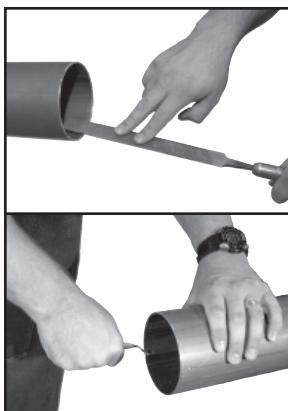
2. Deburr the tube inside diameter using a half-round file or deburring tool. Remove any copper shavings or filings.
