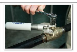
Actuate spring return handle from closed position and insert open end of **5/16" wrench** into gap over Threaded Rod (H). Slowly release handle, allowing space between Connector (G) and Adaptor (C) to be taken up and wrench to be clamped.
