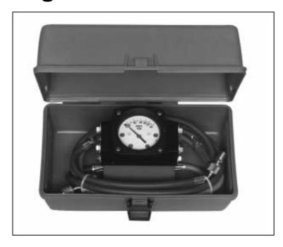
This Test Kit is equipped with a rugged differential pressure gauge with an accuracy of  $\pm$  3-2-3% full scale (ascending) ideally suited for measuring the pressure drop across various types of equipment (i.e. filters, pumps, balancing valves, etc.)
