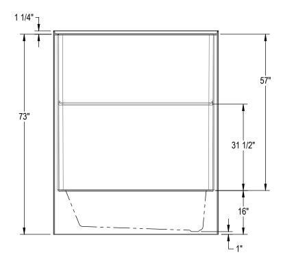
All dimensions are approximate. Structure measurments must be verified against the unit to ensure proper fit.
