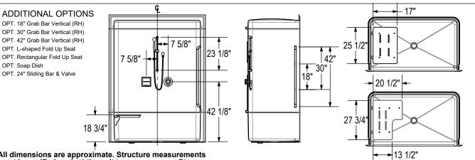
All dimensions are approximate. Structure measurements must be verified against the unit to ensure proper fit.
