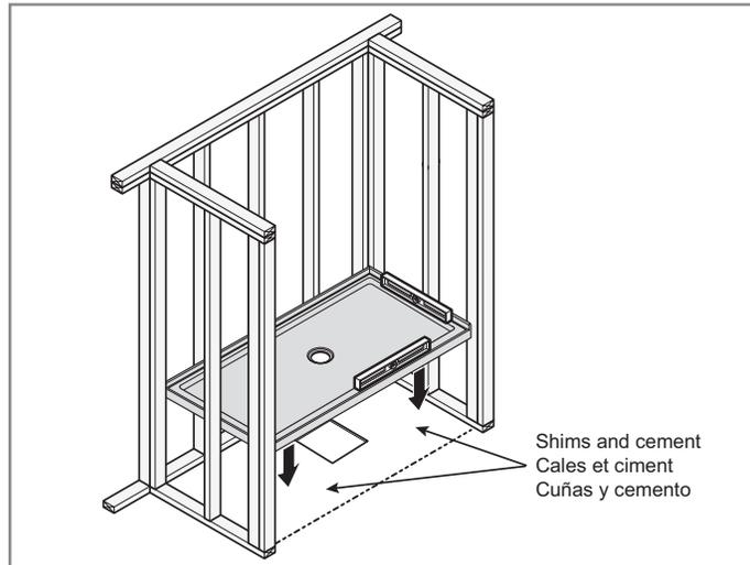
Install the drain by following the manufacturer's directions. Test if the water flows properly: plug the drain, fill the base of the shower with water and unplug the drain to see if the water drains completely and the base is level. If it is not the case, make the appropriate adjustments.
