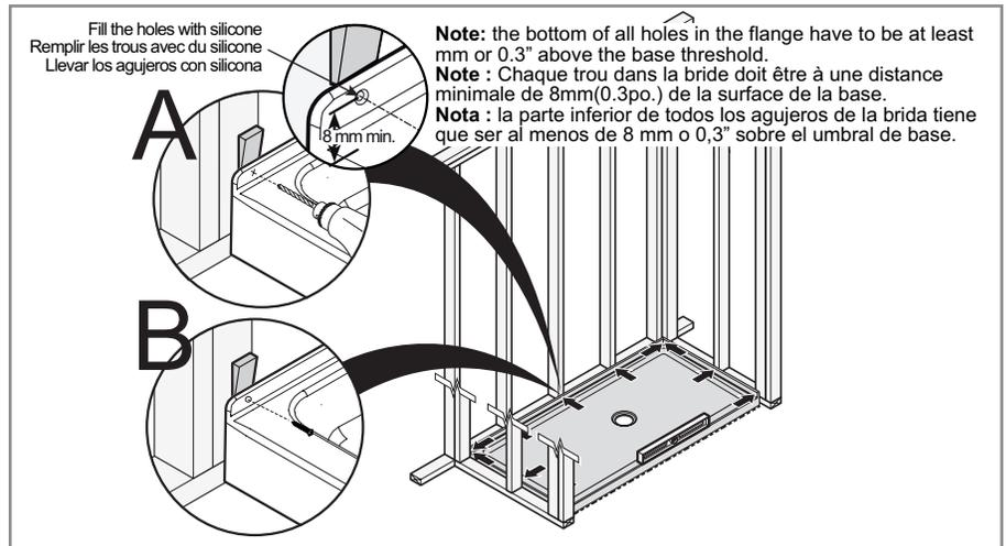
Fasten the base to the studs with # 8 screws by first drilling the mounting flange with a 3/16" bit. If needed, use wooden shims behind the mounting flange to maintain the base in place.
