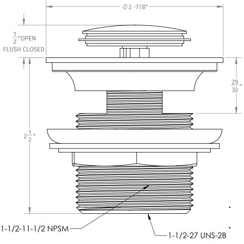
CAN THREAD INTO A 1-1/2 - NPSM STANDARD DRAIN SHOE INTERNAL FEMALE THREADING ALLOWS FOR CONNECTING A 1-1/2" BRASS TUBE (NOT INCLUDED)
